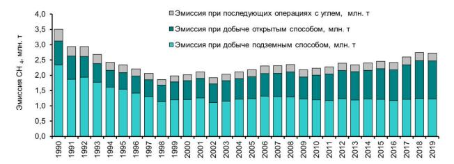
Figure 4. Russian Federation methane emissions in millions of tons per year, from underground coal mining (light blue), open pit coal mining (dark blue) and subsequent operations (gray) [UNFCCC, 2021b, Figure 3.36].
